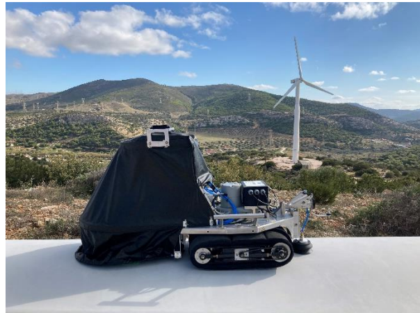
Robotic crawler with vacuum assisted caterpillar tracks and shearography light shield
