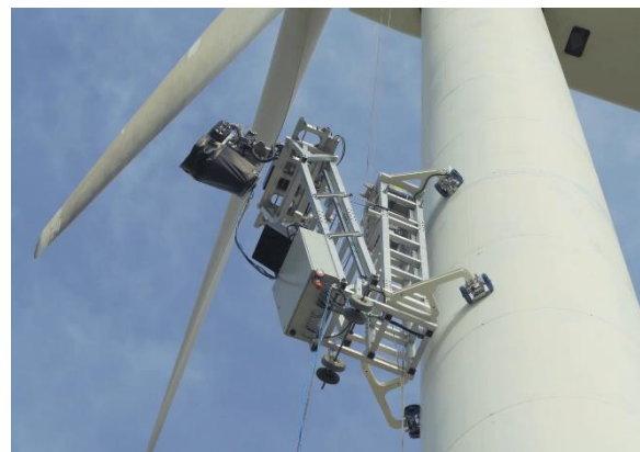
Robotic climber deploying the blade crawler
